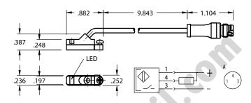
Mechanical Data Housing material Material of sensing face Polyamide Polyamide PVC cable Connection Degree of Protection Rated shock: half-sinus, 30 g, 11 ms Rated vibration environment: 55 Hz, 1mm amplitude, 3 x 30
